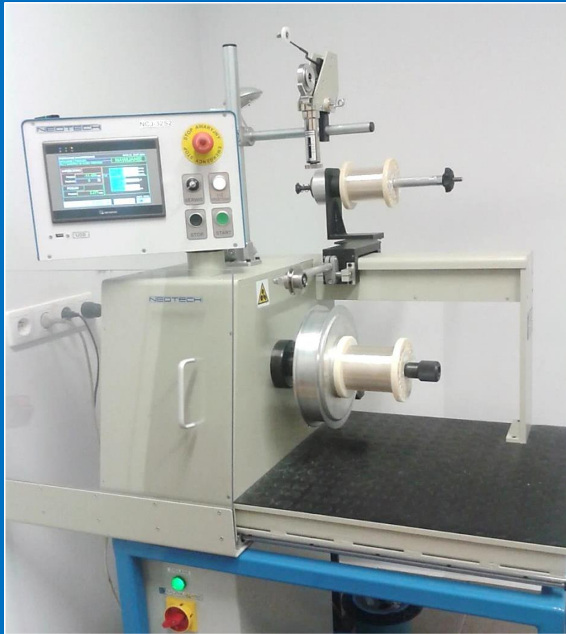
Special set-up for quadrapole-bifilar loop winding
